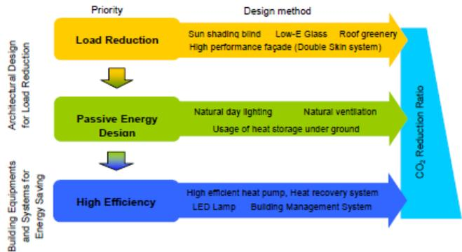
Appendix 2 ‘Low Carbon Measures Along with Cases Examples’ is an attachment of the ‘Concept’. As for Low Carbon Building, six types of case examples are enumerated: ‘Sunlight shading and thermal insulation’, ‘Façade engineering’, ‘Natural ventilation’, ‘Daylight use plus lighting system’, ‘Hybrid of natural ventilation plus air conditioning’ and ‘High-efficient heat source plus heat storage’.
